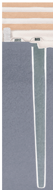
Figure 2. Conventional embedded DRAM (eDRAM) requires a deep-trench capacitor structure in addition to the transistor for each bit-cell. The capacitor trench makes the bit-cell much taller than its width and poses a problem for advanced fabrication processes.
